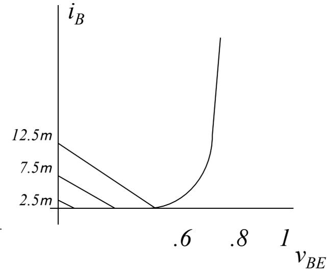
*The Base is biased too low and there is no signal generated in the base and, therefore, the collector circuit.*
