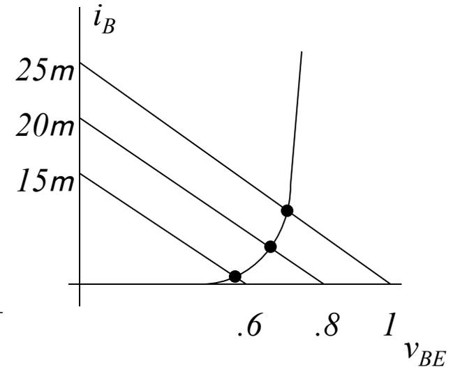
The Collector circuit load line:
